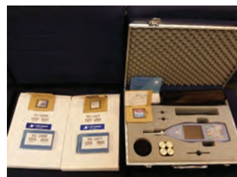
RION Integrating Sound Level Meter & Real-time Analyzer (Department of Civil Engineering)
